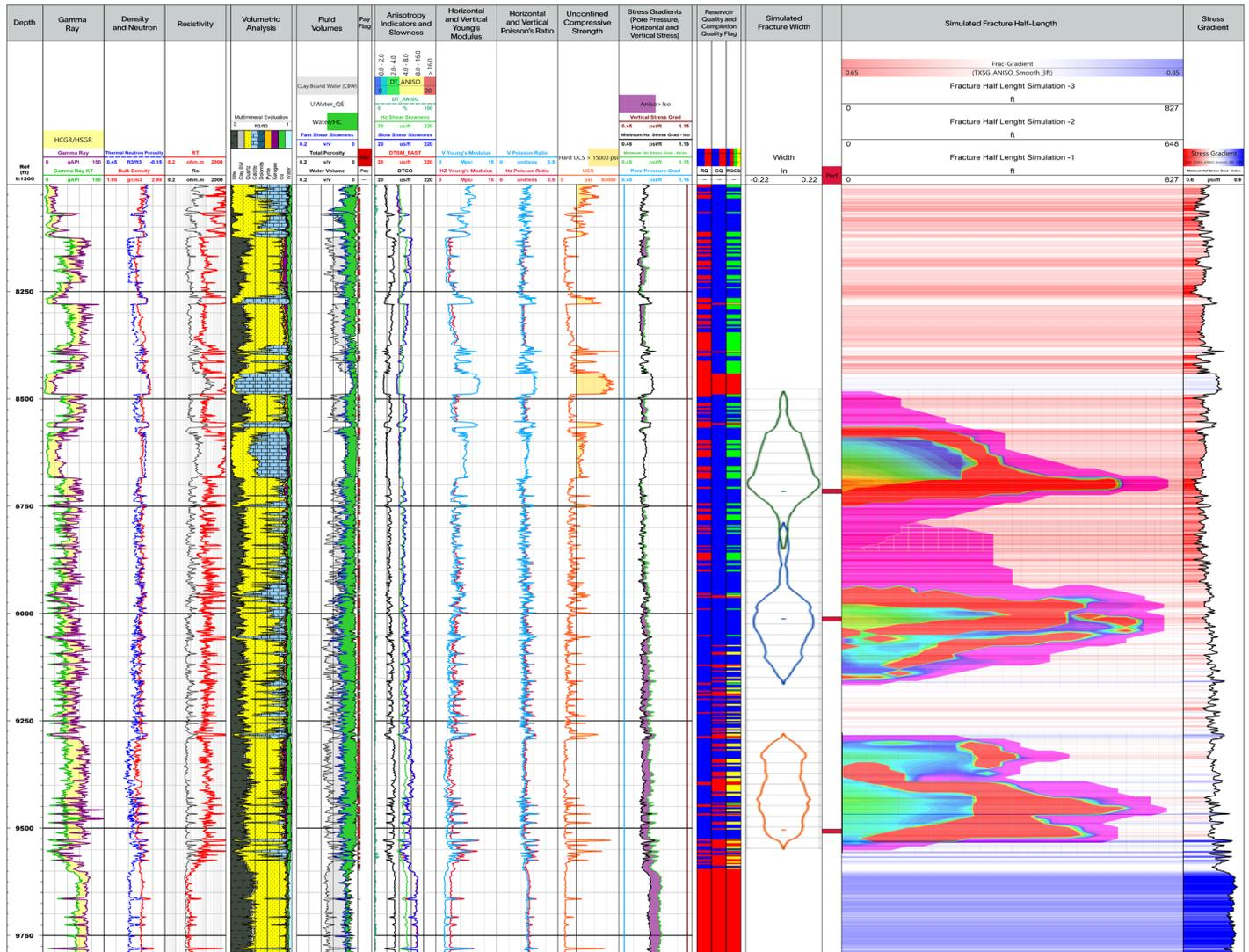
Integrated plot displaying reservoir quality, completion quality, and landing simulation with fracture width and height.
